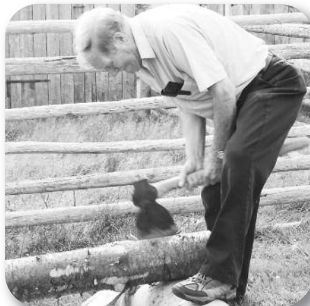
Alan MacLeod (Ailean mac Ruairidh 'ic Aonghais ic Dhòmhnaill 'ic Iain) demonstrates the use of a broad axe at the Highland Village.
